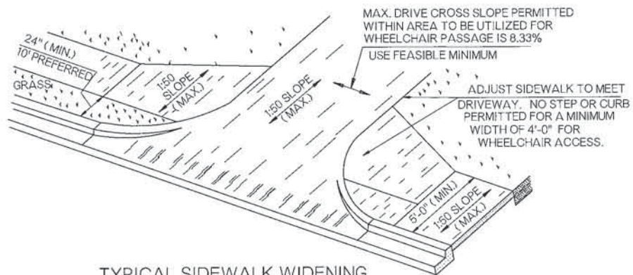
TYPICAL SIDEWALK WIDENING AT DRIVEWAY
